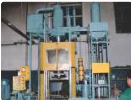
Aluminium die-casting plant
